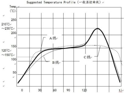
Line A: Used for solder paste soldering.
